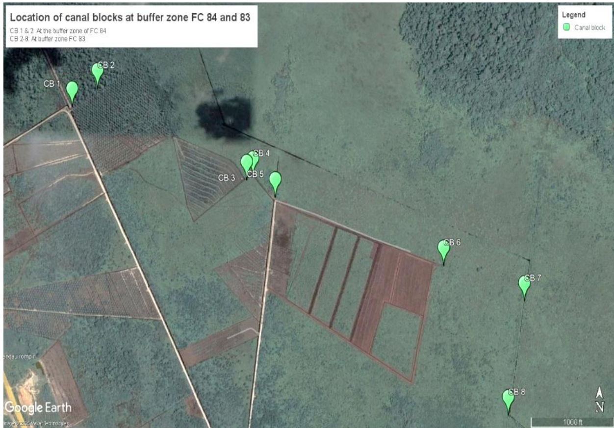
Figure 13. The location of canal blocks / check dams constructed adjacent to the FC 83 and FC 84.
